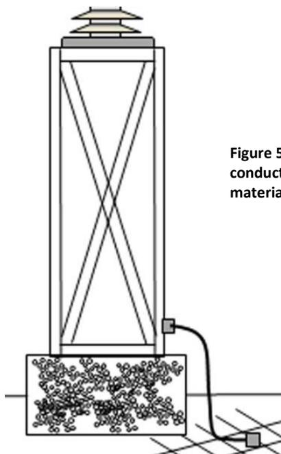
Figure 5: Using the Pedestal as a conductor for the arrester would save on material
